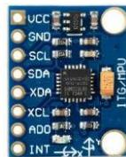
Gambar 6. Sensor MPU-6050.[7]
