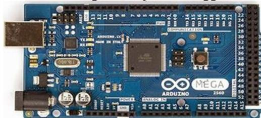
Gambar 1. Arduino Mega 2560.[2]
